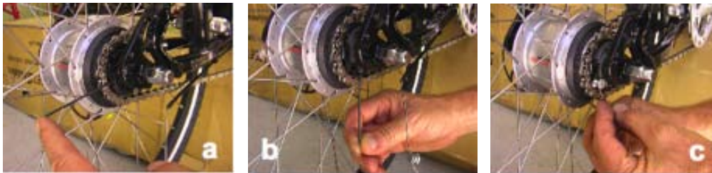
Figure 3-16. Installing the Rear Wheel – ETX 8r (con't)
