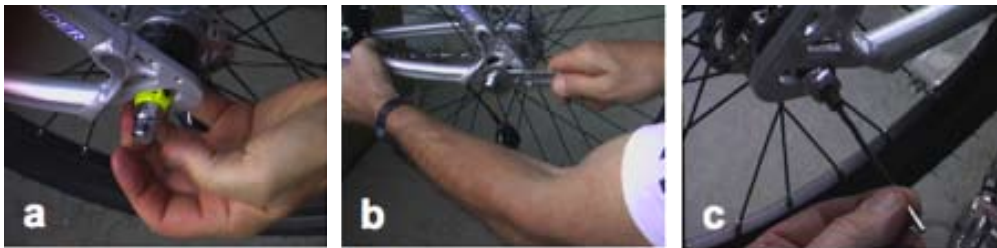
Figure 3-12. Installing the Rear Wheel – ETX 3r (con't)
