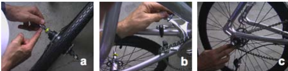
Figure 3-11. Installing the Rear Wheel – ETX 3r (con't)
