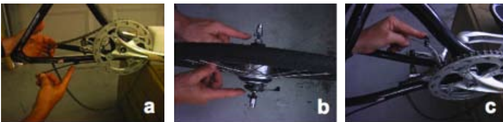
Figure 3-14. Installing the Rear Wheel – ETX 8r
