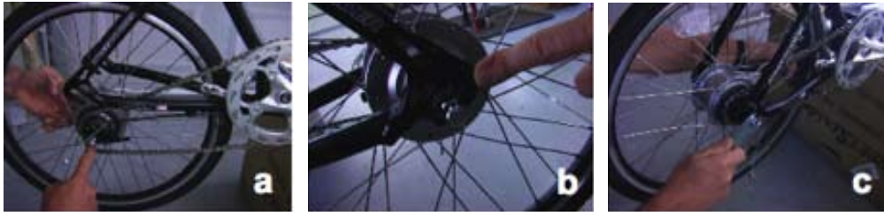
Figure 3-15. Installing the Rear Wheel – ETX 8r (con't)
