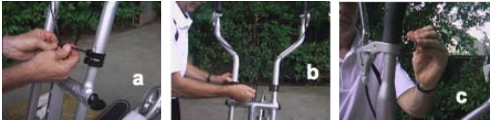
Figure 3-8. Unfolding the Head Tube
