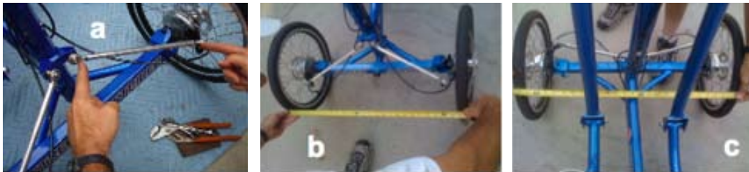
Figure 3-19. Aligning the Front Wheels
