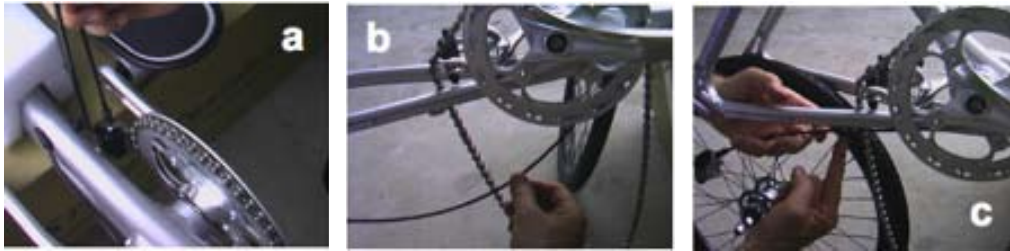
Figure 3-10. Installing the Rear Wheel – ETX 3r (con't)
