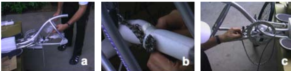
Figure 3-9. Installing the Rear Wheel – ETX 3r
