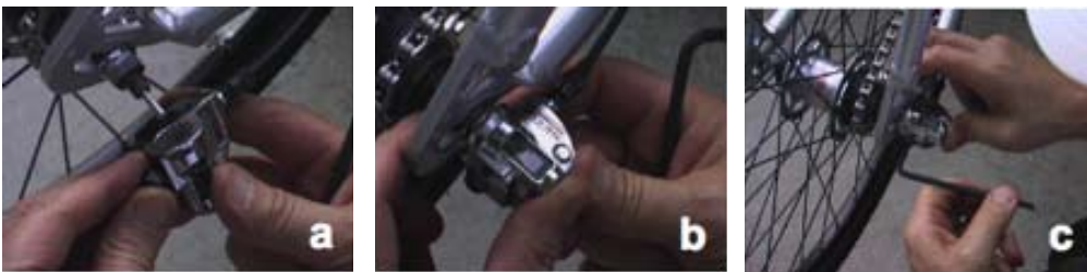
Figure 3-13. Installing the Rear Wheel – ETX 3r (con't)
