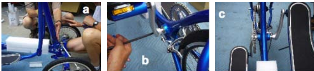
Figure 3-23. Folding the ETX for Transportation or Storage
