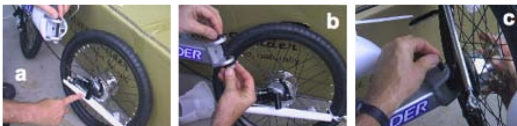
Figure 3-3. Attaching the Two Front Wheels
