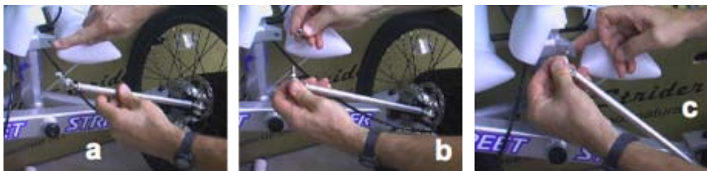
Figure 3-4. Attaching the Two Front Wheels (con't)
