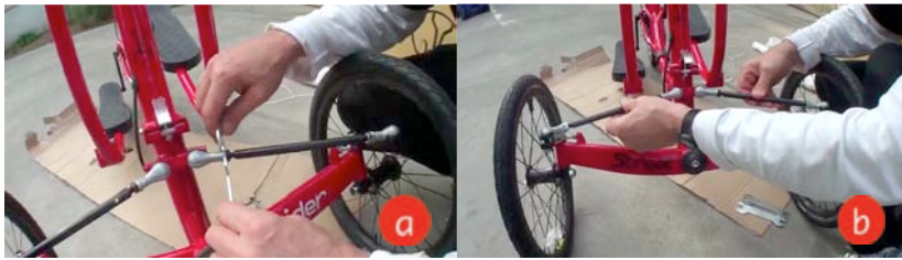
Figure 3A-11 a, b. Aligning the front wheels
