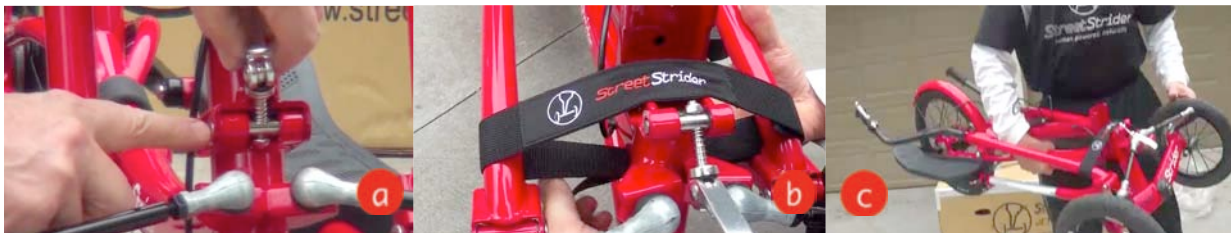
Figure 3B-7 a, b, c. Folding the JET for transport or storage (cont'd)
