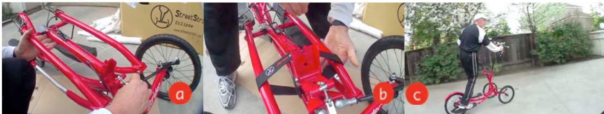
Figure 3A-13 a, b, c. Folding and unfolding the Eclipse (con't)
