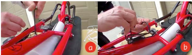
Figure 3A-6 a, b. Attaching the bottle cage
