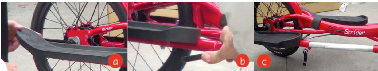
Figure 3B-6 a, b, c. Folding the JET for transport or storage
