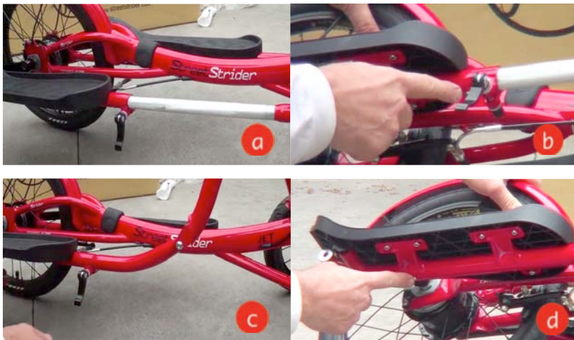
Figure 3B-3 a, b, c, d. Collapsing the telescoping strider ski
