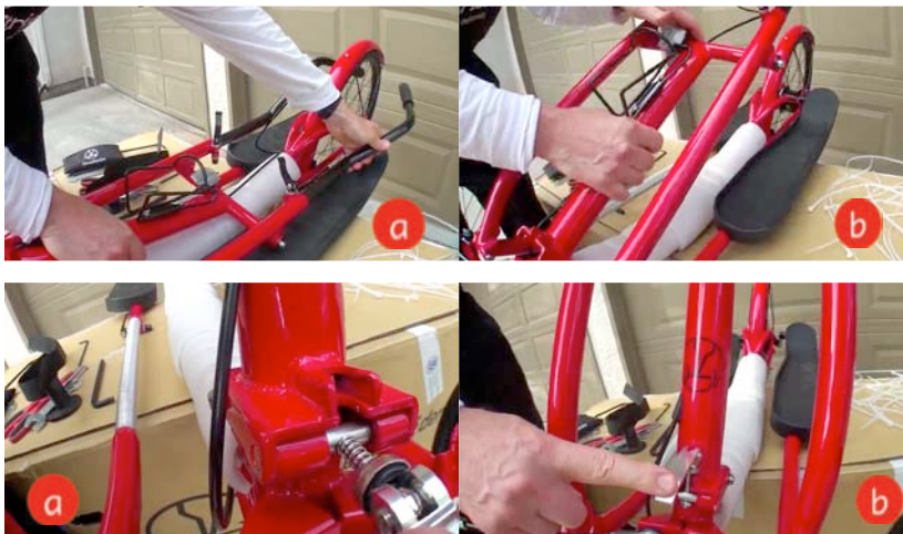
Figure 3A-7 a, b, c, d. Unfolding the head tube
