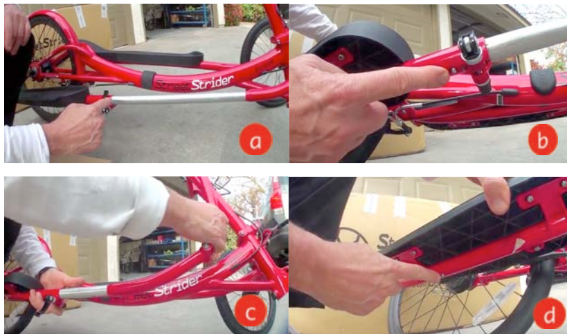
Figure 3A-8 a, b, c, d. Collapsing the telescoping strider ski
