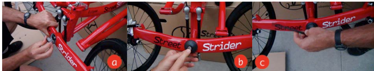
Figure 3A-3 a,b,c. Attaching the front end (con't)
